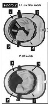
in the helmet's suspension ring. The position of the headband in these four tabs determines the position of the headband on your head. There are 6 numbered positions on each headband mounting tab whereby the headband can be moved inward or outward. The factory setting is for the average-size head.
