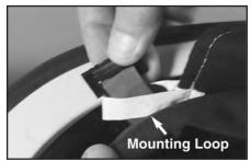
as when removing ear covers. This time, however, slip the white mounting loop back over the suspension mounting tab. Make sure the white tab material does not interfere with the suspension tab fitting back into its slot. Then snap the suspension tab into place with your thumb. Continue, one tab at a time, for the remaining headband mounting tabs 2, 3, and 4 and the suspension mounting tab 5.
