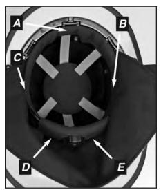
PLUS Models – The one-piece brow pad/comfort cap (headband cover) is held in place with hook tape at positions A, B, and C. The ratchet cover is held in place with hook tape at positions D and E.
