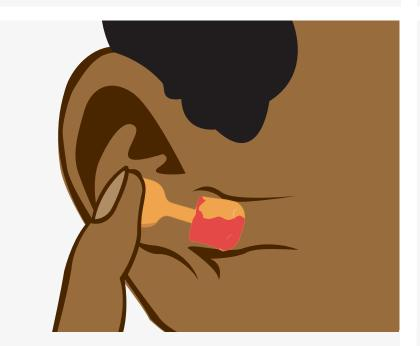
Insert earplug so foam tip is well inside the ear canal. Use a gentle rocking motion while pushing earplug into ear canal to ensure a deep fit.
