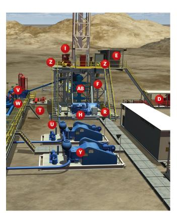
Mud pump stroke count, position sensing, or on/off
