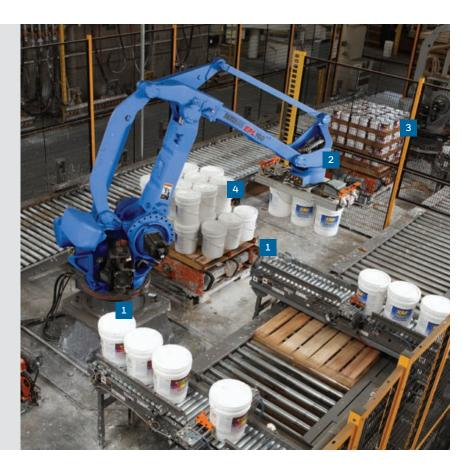
can redesign the existing end effector or create a new one to meet revised packaging configuration needs. The flexibility that modular tooling provides means that palletizing robots can be relocated to new lines or facilities that handle different styles of packaging or increased line speeds, whether it's case, pail, bundle or bag, in-case, row or layer quantities.
