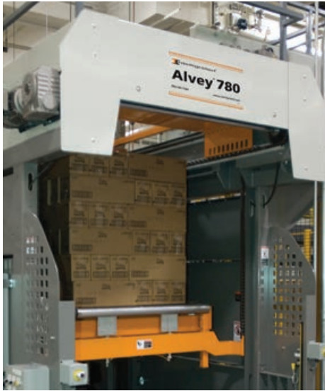
The Alvey 780 palletizes higher-speed SKUs at a rate of up to 37 cartons per minute.
