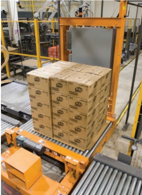
A Honeywell Intelligrated laser-positioned, rail-running transfer car brings completed loads from the robots to a turn-table that directs them to the stretch wrapper.
