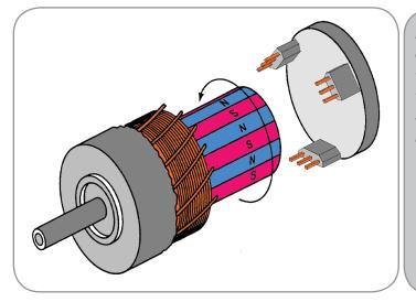
BLDCs use electronic commutation to control the power distribution to the motor, using Hall-effect sensors to measure the motor's position.
