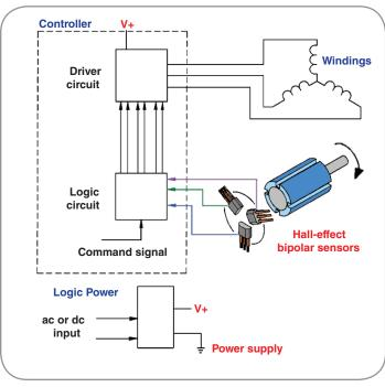
Bipolar Hall-effect sensors are used in BLDC motors to detect the position of the rotating magnet. In this example, an eight-pole motor with a three-phase winding uses three bipolar latching Hall-effect sensors.
