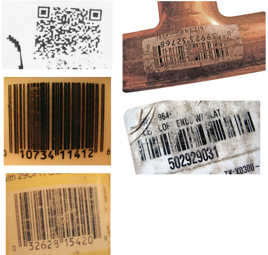
FIGURE 1. DAMAGED OR DISTORTED BARCODES
