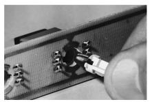
Insert the LED/PWB receptacle assembly through a hole in the printed wiring board.
