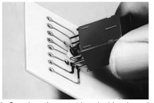
Seat housing on printed wiring board, with LED projecting into hole at the base of the housing.
