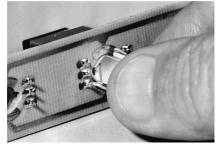
A ½-turn applied clockwise to the receptacle locks it in the printed wiring board and establishes the electrical connection.
