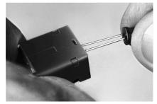
Assemble LED to MML44 indicator, with the LED terminals protruding through assembly slot in the middle of housing base.
