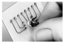
Assemble stand-off spacer to LED terminals and seat on printed wiring board.
