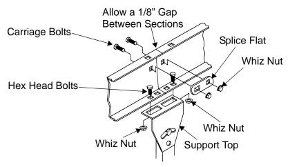
Figure G - 1 Standard Floor Support Assembly
