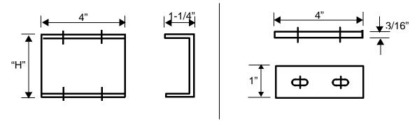
Figure G - 5 Connector Channel
