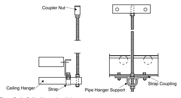
Figure G - 2 Ceiling Hanger Installation
