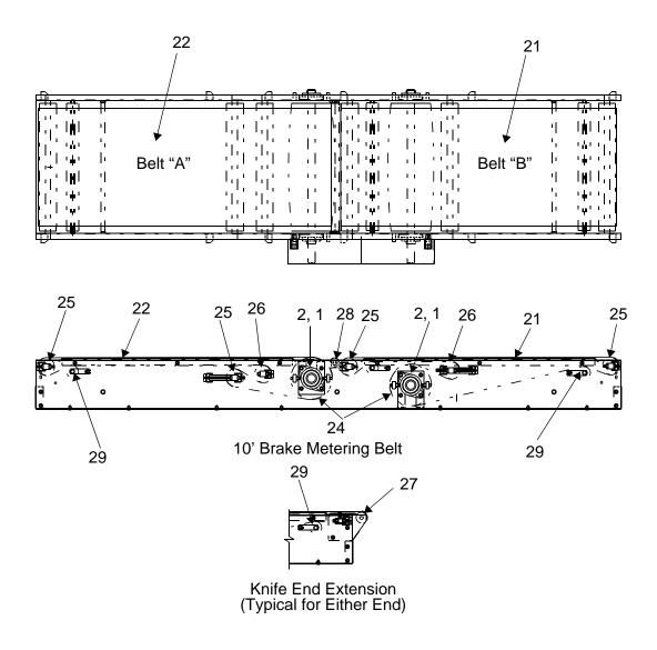
Figure I - 1 Brake Metering Belt - Top and Side View, and Knife End Extension
