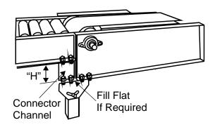
Figure G - 4 Connector Channel
