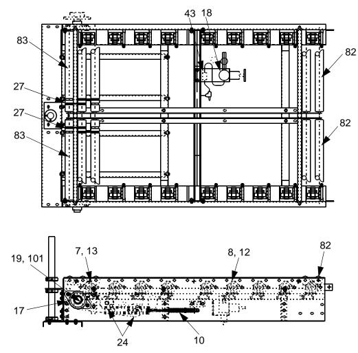
Figure I - 1 Powered Roller Merge Drive Unit
