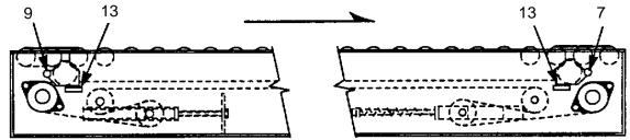
For DR Section Clutch (13) Only - Select RH/LH assembly that is opposite the mounting side Example: Use LH assembly when mounting on RH side of conveyor.
