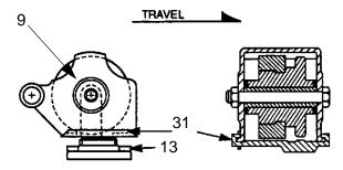
Figure I - 9 Take-Up Section Clutch Components
