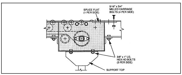
Figure G.23 - Power Transfer Unit Connection
