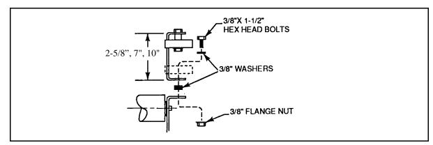
Figure G.36 - Mounting Wheel Face Side Guide
