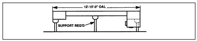
Figure G.8 – 12'-15'-0" OAL Shipped Fully-Assembled Attach Three Supports
