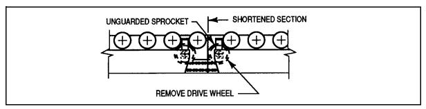
Figure G.54 - Removal of Unguarded Drive Wheel/sprocket
