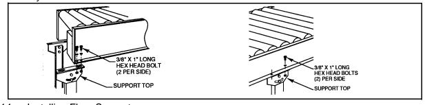
Figure G.14 – Installing Floor Supports
