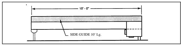
Figure G.32 - Model PRS Conveyor 10'-0" Long (shipped from the factory as complete unit)
