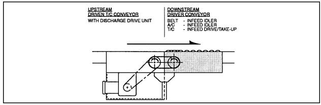
Figure G.63 – Discharge Drive Unit, Direct-Rotation PTO Infeed Drive Unit, Direct-Rotation PTO - (not shown)
