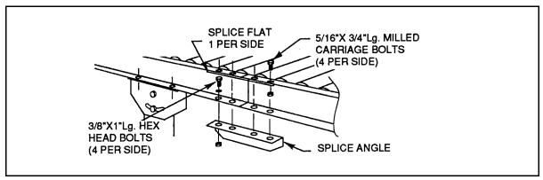
Figure G.5 – Use Splice Angle Assembly at Splice Point When Floor Support or Ceiling Hanger Must Be Offset
