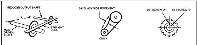
Figure G.60 – Sprockets must be Aligned.
