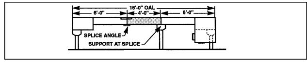
Figure G.9 – 16'-0" OAL Shipped as Components Attach Three Supports and One Splice Angle
