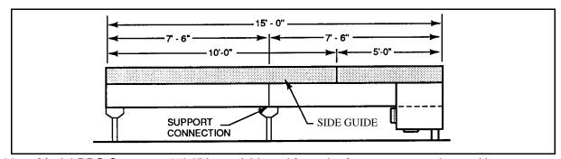
Figure G.33 - Model PRS Conveyor 15'-0" Long (shipped from the factory as complete unit)
