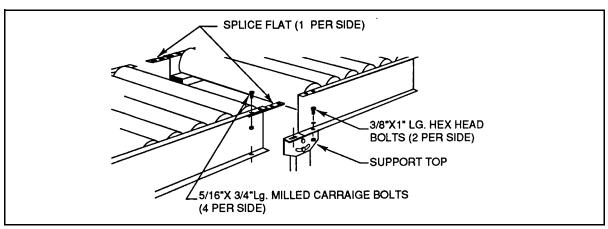
Figure G.4 - Splice Intermediate Sections Together
