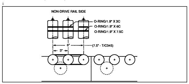
Figure G.57 - Order O-Rings/Grooved Rollers as Required for Conveyor With ("W") and T/C Series
