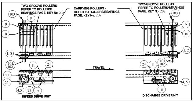
Figure I - 1 — Infeed Drive Units and Discharge Drive Unit
