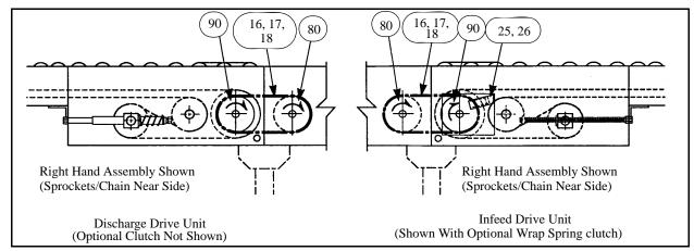
Figure I - 7 — Discharge Drive Unit (Left) and Infeed Drive Unit (Right) with Power Take-Off Units
