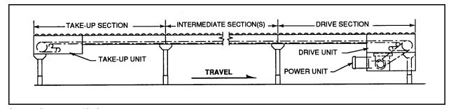
Figure G.1 - Style 1, T/C Conveyor with Discharge End Drive Unit
