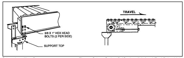
Figure G.2 - Installing Supports
