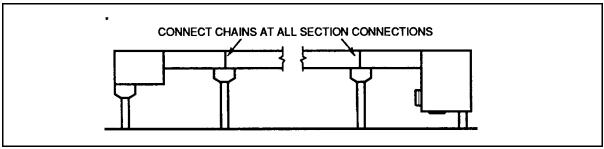
Figure G.37 - Style 1 - T/C Straight Conveyor
