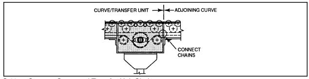
Figure G.41 - Connect Curve and Transfer Unit Chains
