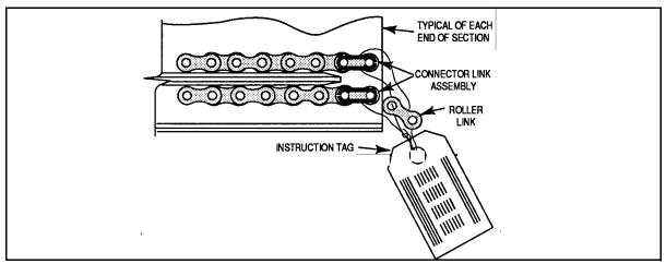
Figure G.38 - Instruction Tags on Connector Link Assembly
