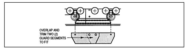
Figure G.56 - Lengthened Guard Segment
