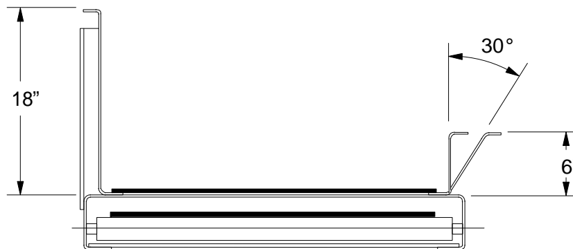
Figure B - 10 Vertical Side Guides
