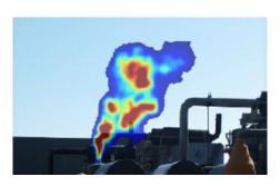
A release of hydrocarbon gas and its concentration is clearly shown with a CGI camera.
