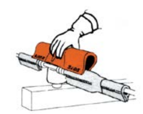
Remove by "rolling off" sideways.
